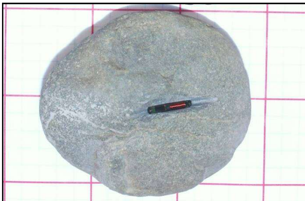
PIT tag inserted into a cobble
