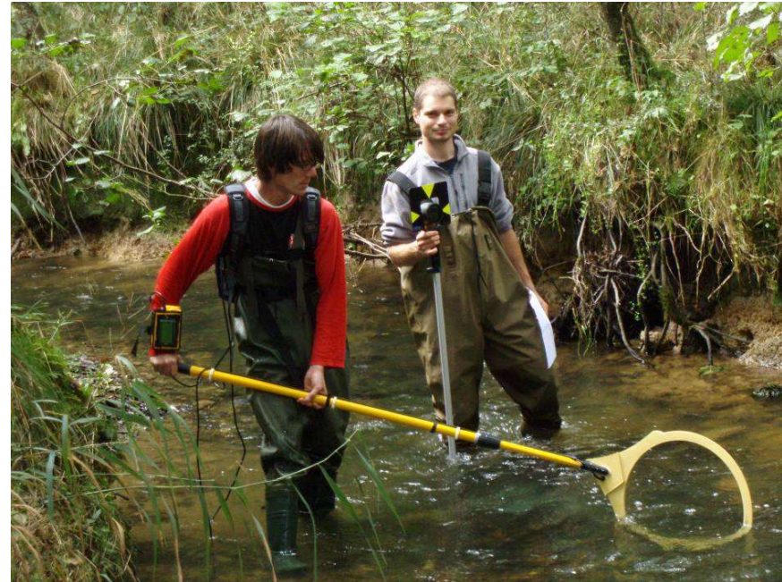
Field survey with loop induction antenna and reading unit
