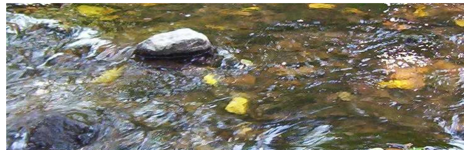
Painted tracer gravels with PIT tag
